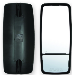
24V MIRROR HEAD Suits Volvo FL, FE & FM excluded Series 1 (Electric & Heated) 480 x 214mm • 16-28mm Clamp
