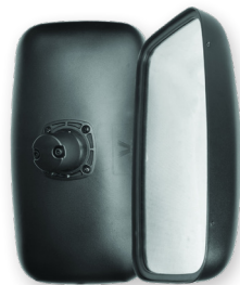
UNIVERSAL MIRROR HEAD Flat Glass • 415 x 225mm 16-28mm Clamp • Suits Hino F Series & Isuzu F Series up to 2006
